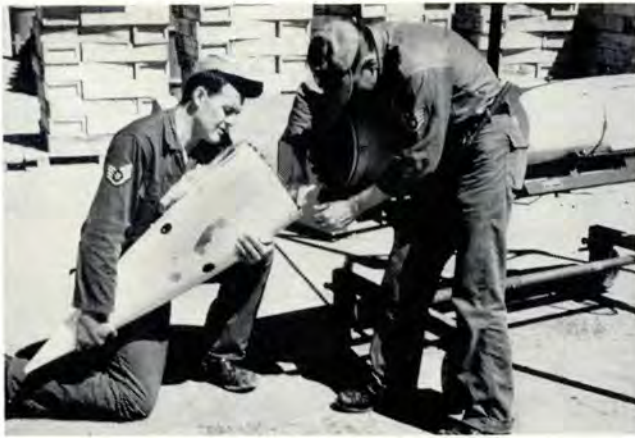
Steps in preparing the GAM-83A for action are shown in this picture sequence. Top left, two crewmen connect nose section to the rest of missile; simple lock ring holds missile together. Top right, MJ-1 lift is shown in use, lifting missile from its cradle after arriving in the aircraft loading area. Lower left, ground crewman makes electrical check on launcher prior to loading BULLPUP on the F-100, and in last photo the ground crewman loads missile on F-100 launcher with the MJ-1 lift truck. Wings and canards are attached after BULLPUP is mated to the aircraft.
