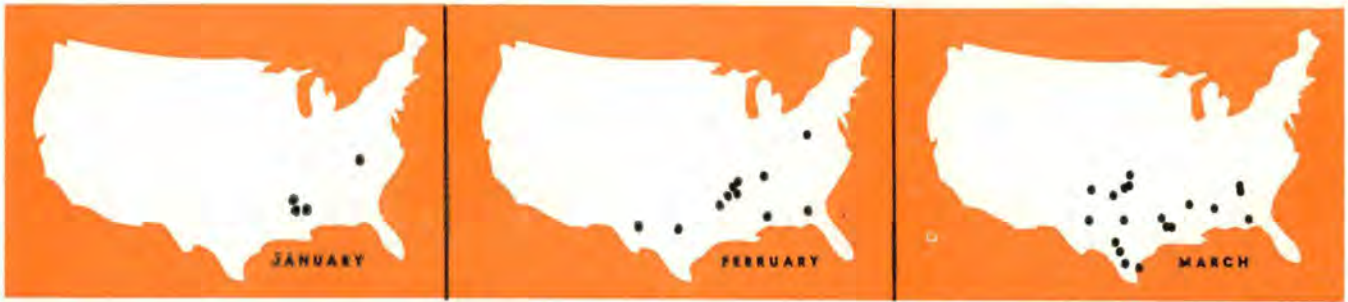
Encounters with damaging hail aloft reported by aircraft illustrate the seasonal movement beginning around the first of the year in the south-east and gradually moving northwest, receding during the fall months. If you're unlucky and get clobbered, report it via Channel 13.
