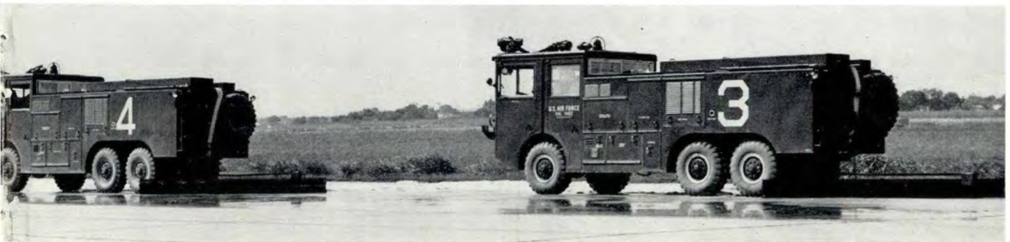
A king-size squeegee makes an excellent foam-remover. Details of simple device are shown in picture at left. At right, it's attached to fire truck. Quick removal of foam is shown in lower photo as trucks in tandem, each cutting a 15-foot swath, move swiftly down the runway. Four of these units can move a 20-foot wide strip 60 feet from centerline in about fifteen minutes.
