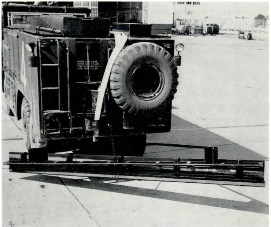
A king-size squeegee makes an excellent foam-remover. Details of simple device are shown in picture at left. At right, it's attached to fire truck. Quick removal of foam is shown in lower photo as trucks in tandem, each cutting a 15-foot swath, move swiftly down the runway. Four of these units can move a 20-foot wide strip 60 feet from centerline in about fifteen minutes.
