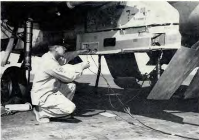
Steps in preparing the GAM-83A for action are shown in this picture sequence. Top left, two crewmen connect nose section to the rest of missile; simple lock ring holds missile together. Top right, MJ-1 lift is shown in use, lifting missile from its cradle after arriving in the aircraft loading area. Lower left, ground crewman makes electrical check on launcher prior to loading BULLPUP on the F-100, and in last photo the ground crewman loads missile on F-100 launcher with the MJ-1 lift truck. Wings and canards are attached after BULLPUP is mated to the aircraft.
