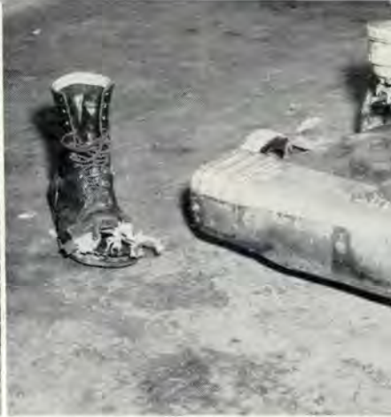
In the springtime a man's fancy turns to other things. But it shouldn't if you're maneuvering a power mower as these pictures illustrate. The imprudent airman can easily be shot down in his own backyard if he isn't careful. First picture shows position of shoe if operator were standing in front of mower; center, damage inflicted by blade. Probable position of shoe at the time of the accident is shown in last photo.
