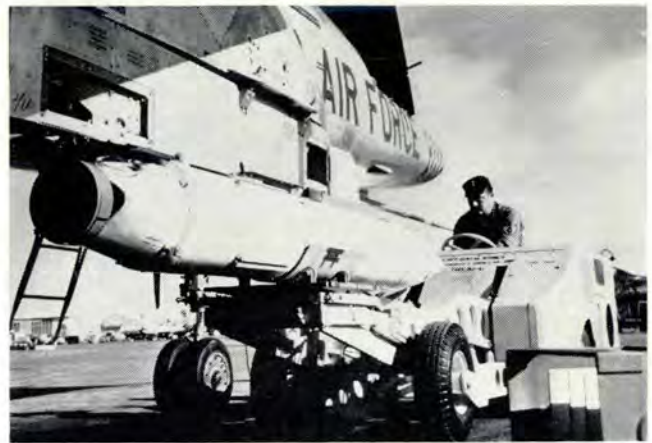
Steps in preparing the GAM-83A for action are shown in this picture sequence. Top left, two crewmen connect nose section to the rest of missile; simple lock ring holds missile together. Top right, MJ-1 lift is shown in use, lifting missile from its cradle after arriving in the aircraft loading area. Lower left, ground crewman makes electrical check on launcher prior to loading BULLPUP on the F-100, and in last photo the ground crewman loads missile on F-100 launcher with the MJ-1 lift truck. Wings and canards are attached after BULLPUP is mated to the aircraft.
