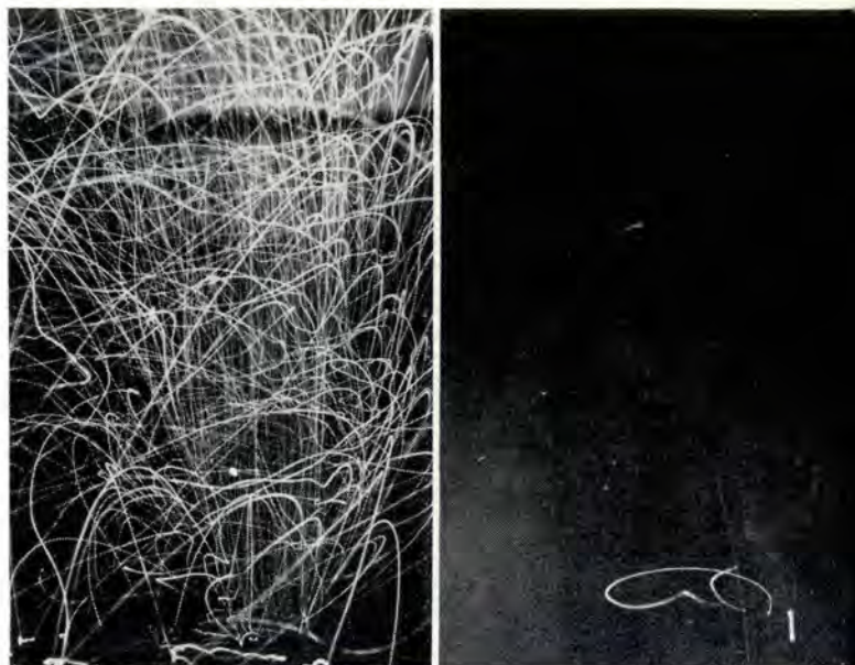
Effect of spark arrestor is shown here. Fourth of July-like display, left, gives idea of hazards resulting from sparks emitted by internal combustion engines. Arrestor nearly eliminated this hazard, right.
